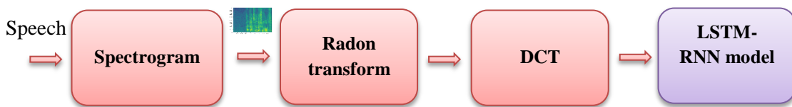
Fig. 4.16 Proposed ASR system based on Radon features.
